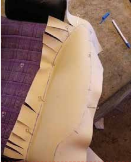
When marking out new templates, pin a similar scrap piece of material to each panel you're marking out.
