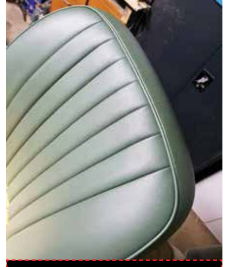
Sew piping to the box border first and then sew it to the pleats so that it floats over the pleats, keeping the piping tight and looking good.
